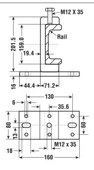
System Max. Static Radial Load = 16.5 KN / 1.8 US Ton-Force SHOWN PROFILE RAILS, System Max. Static Axial Load = 5.5 KN / 0.6 US Ton-Force
