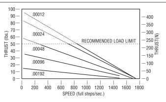
Size 17 Stepper Motor with 5.54mm (0.218") Screw
