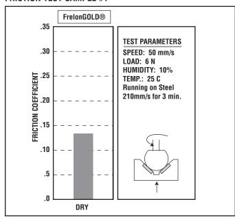
For example, dry running virgin (unfilled) Teflon® on steel's coefficient of friction (c.o.f.) is approximately .1 while filled Teflon's c.o.f. can range from .125 to .4 depending on the fillers used. By comparison, however, the virgin Teflon will wear at a much greater rate.
