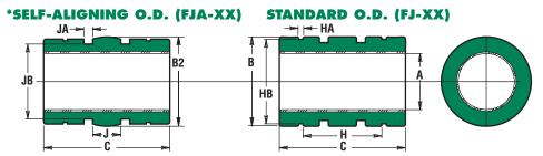
\*Except for the O.D. bearings with the self-aligning feature have the same dimensions and tolerances as the standard bearing. There is a spherical crown on the O.D. to create the self-aligning feature. They are for use in a straight bore housing. Add an "A" to the part number per the example. More information on self-aligning bearings is on page 41-42.
