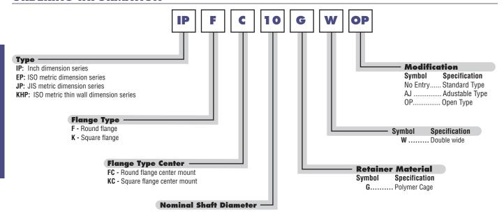
NOTE: Precision of inscribed circle diameters and outside diameters for the clearance adjustable type (...-AJ) and the open type (...-OP) indicates the value obtained before the corresponding type is subjected to cutting process.
