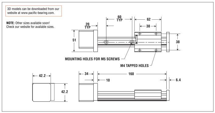
**NOTES:** Maximum length for lead screw driven MR is 640mm. Standard and cut-to-length rail ends are NOT coated. Fully coated rails are available upon request.
