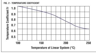
**NOTES:** Maximum temperature of plastic retainer 212°F or 100°C. Maximum temperature 176° per Table 6.
