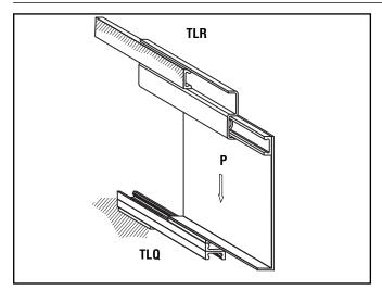
The Redi-Rail® Precision Drawer Slides & Redi-Rail® Compact Precision Drawer Slides systems are the world's only telescopic rail system for complete extension, based on precision rollers and hardened raceways and with incorporate self-aligning feature (RDR series).
