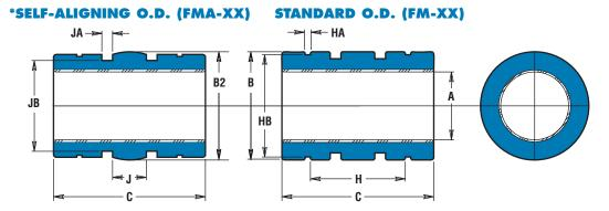
\*Except for the O.D., bearings with the self-aligning feature have the same dimensions and tolerances as the standard bearing. There is a spherical crown on the O.D. to create the self-aligning feature. They are used in a straight bore housing. Add an "A" to the part number per the example. More information on self-aligning bearings is on pages 41-42.
