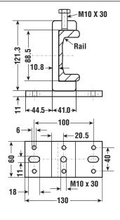
WHEN USED WITH System Max. Static Radial Load = 7.2~KN / 0.8~US Ton-Force SHOWN PROFILE RAILS, System Max. Static Axial Load = 2.4~KN / 0.3~US Ton-Force
