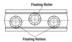
The "Floating" slides contain only floating rollers, three or five in total. The contact areas with the raceways only provide for radial load and Mz capacities, thus allowing for axial movement and a simultaneous slight rotation of the slide to offer axial and longitidinal compensation, while maintaining original preload and same precise and smooth straightline movement.
