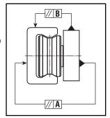
When the RRT-rail is loose, it may result slightly curved. However, this does not give rise to any problem of alignment, once the rail is properly fixed.
